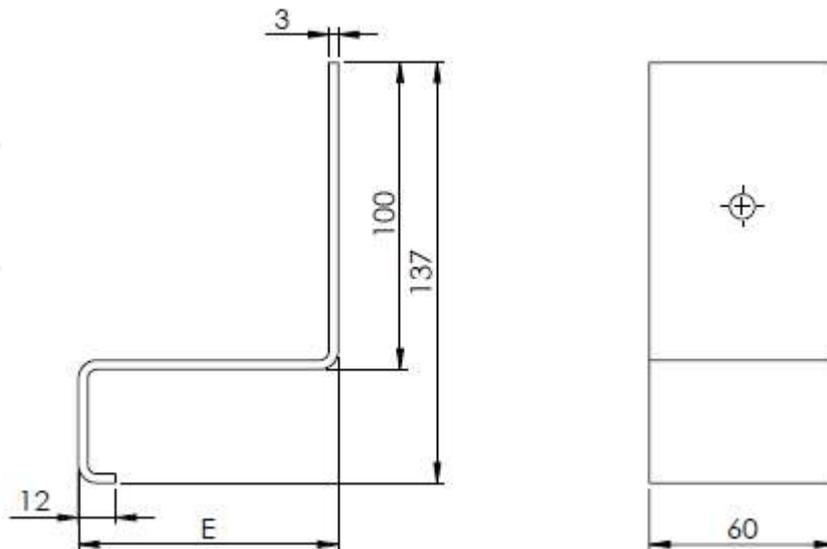
Figure 8. Proposed dimensions of mounting brackets for installation in a ceiling
