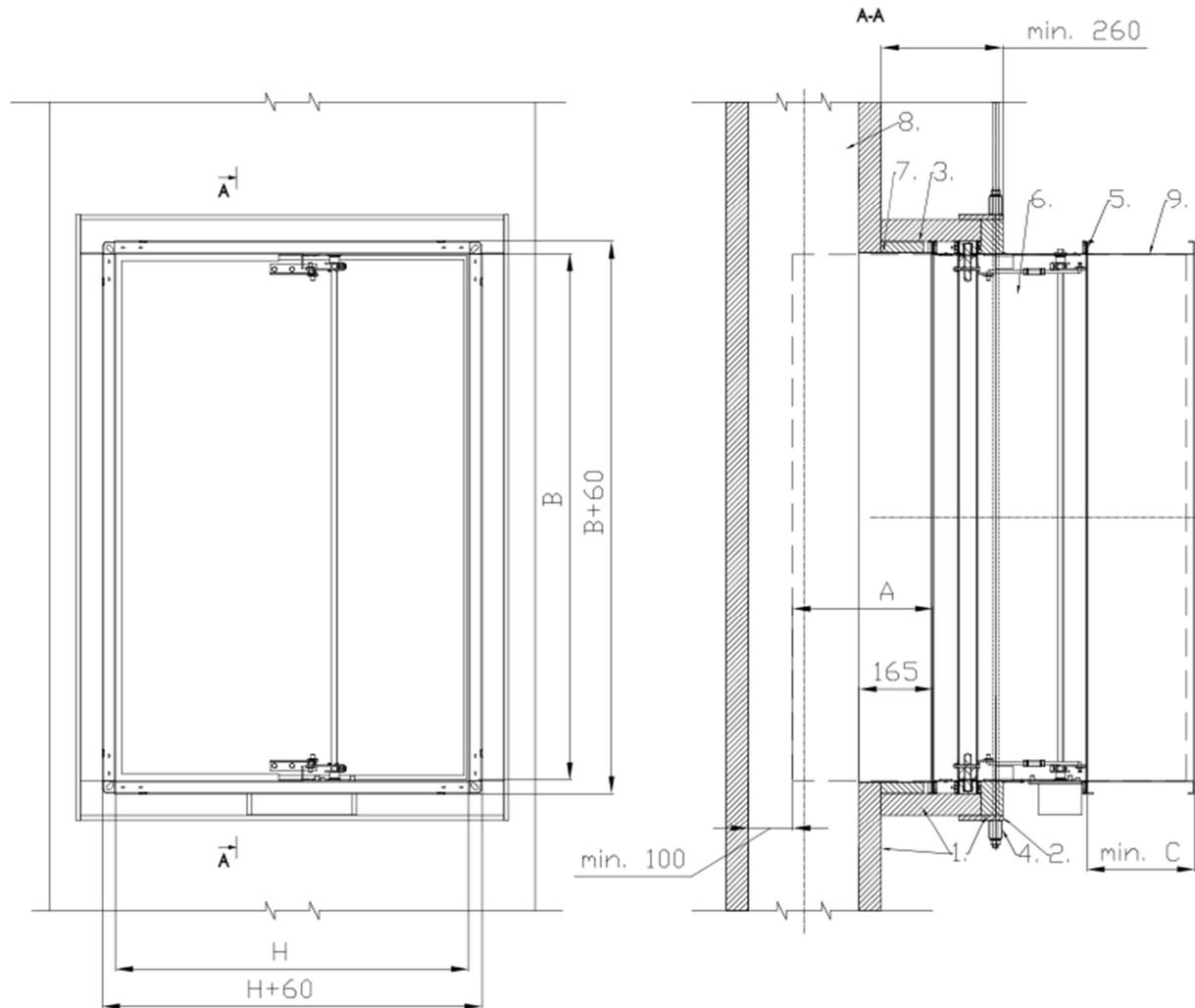
Figure 9. Installation method of dampers on the tee
