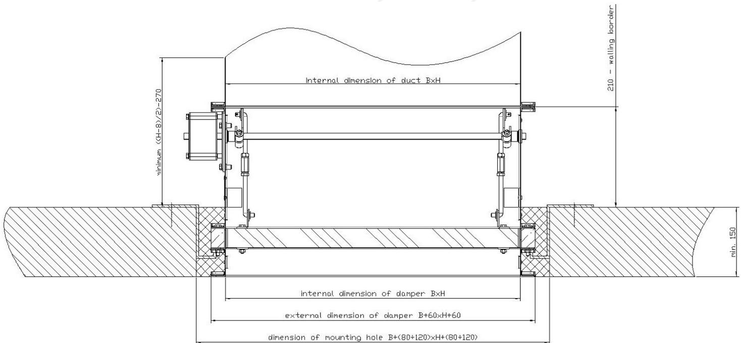
Figure 6. Installation method of fire dampers KWP-O in ceiling with a fire ventilation duct with sealing of cement mortar
