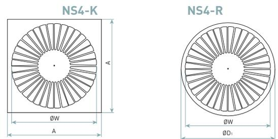
Figure 1. NS4 front panel dimensions.
