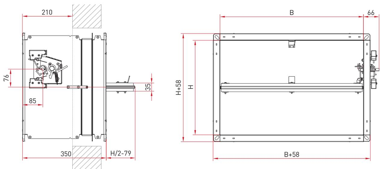
Figure 2. KWP-LS damper (with a spring mechanism).
