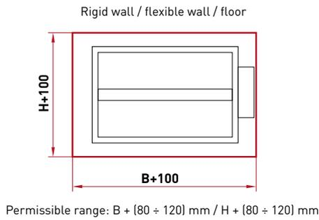
Figure 3. Openings required for the KWP-L damper.
