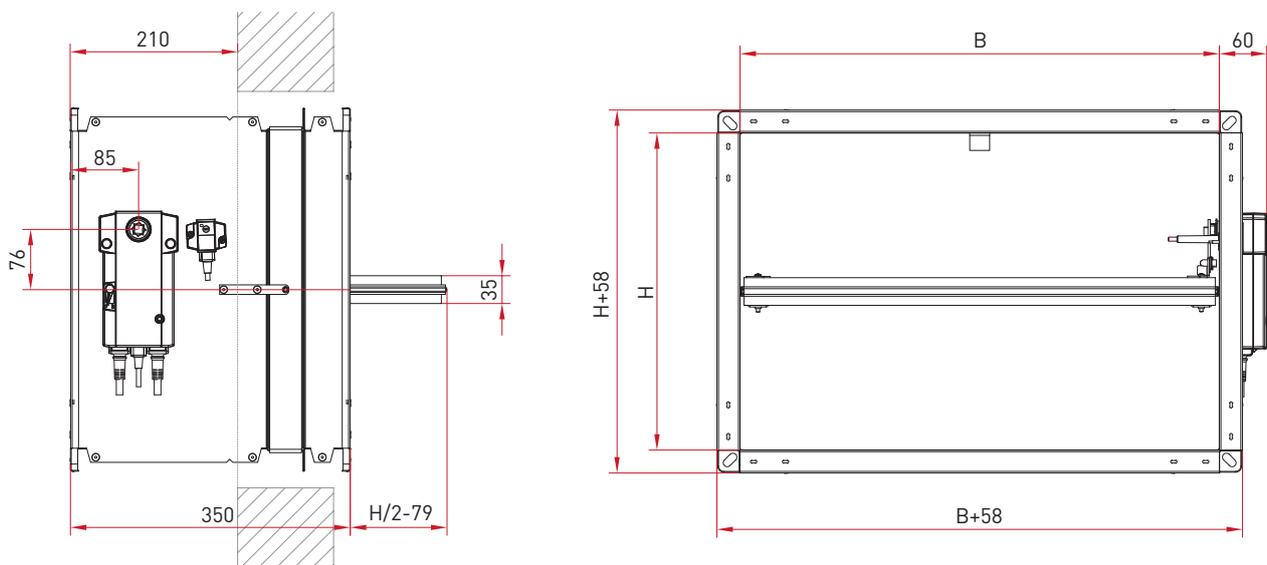
Figure 1. KWP-LE damper (with an electric actuator).
