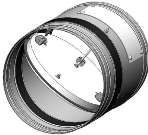
Figure 30. Inspection opening in KTM-O damper
