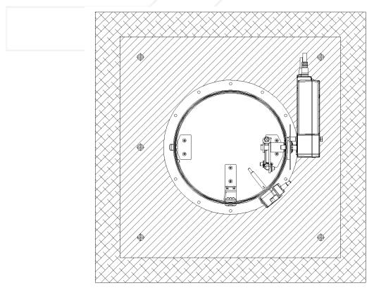
Figure 9. Installation method of fire dampers KTS-O in flexible wall with horizontal rotation axis of baffle
