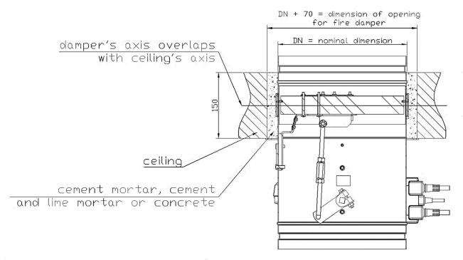
Figure 1. Installation method of fire dampers KTS-O in ceiling
