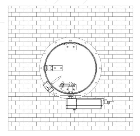
Figure 5. Installation of KTS-O in rigid wall construction with vertical axis of rotation of the damper.
