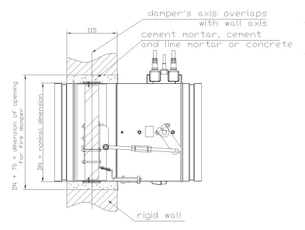
Figure 3. Installation of KTS-O in rigid wall construction with 115 [mm] wall thickness.
