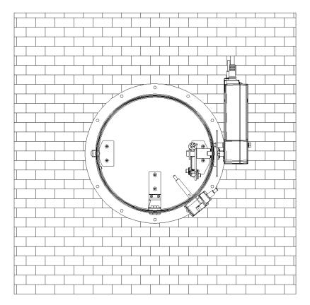
Figure 4. Installation of KTS-O in rigid wall construction with horizontal axis of rotation of the damper.
