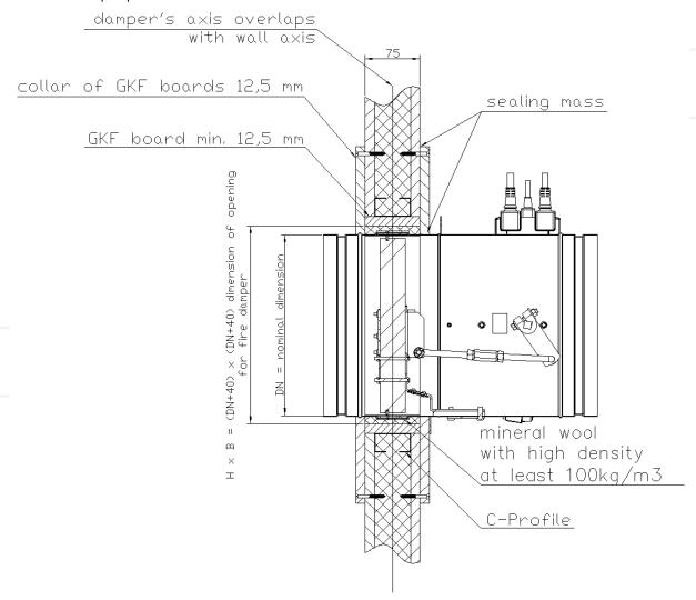
Figure 7. Installation of KTS-O in flexible wall construction with 75 [mm] thickness
