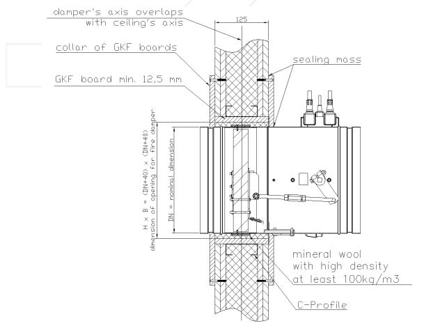
Figure 11. Installation method of fire dampers KTS-0 in flexible wall with 125 [mm] thickness
