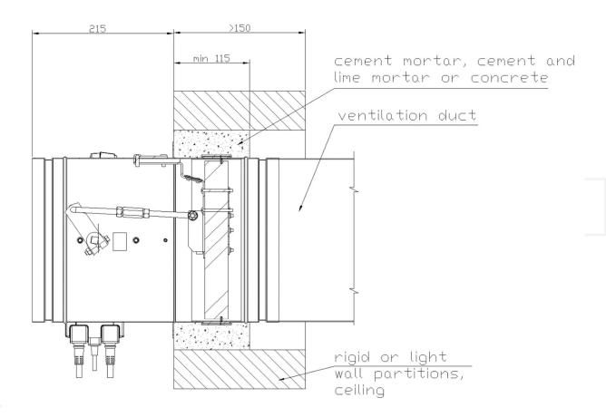
Figure 12. Installation method of fire dampers KTS-O in high wall thickness constructions
