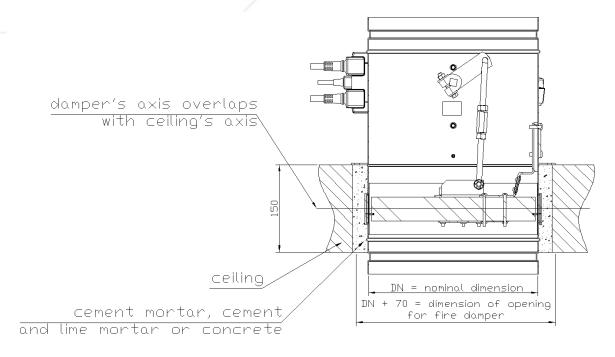
Figure 2. Installation method of fire dampers KTS-O in ceiling
