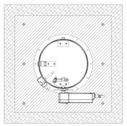
Figure 10. Installation method of fire dampers KTS-O in flexible wall with vertical rotation axis of baffle
