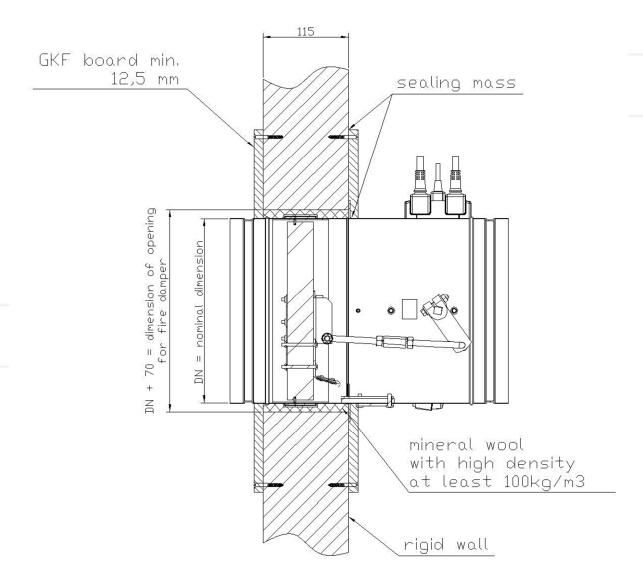
Figure 6. Installation of KTS-O fire dampers in rigid wall
