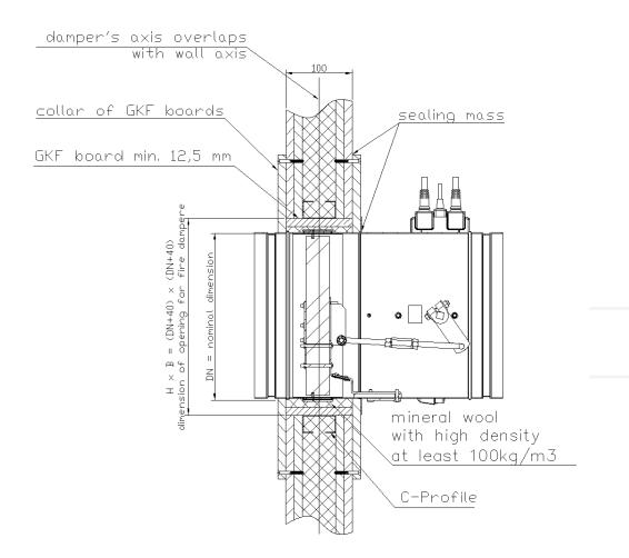
Figure 8. Installation method of fire dampers KTS-O in flexible wall with 100 mm thickness
