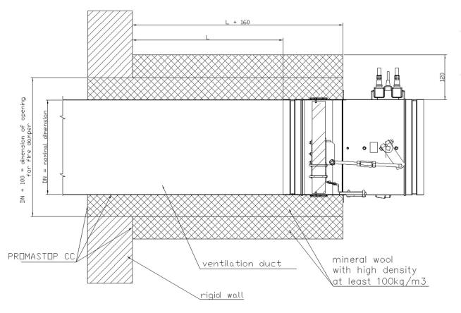
Figure 13. Installation method of fire dampers KTS-O away from wall constructions
