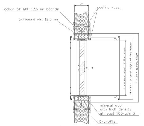
Figure 10. Installation method of fire dampers KWP-L in flexible wall 100 mm thick
