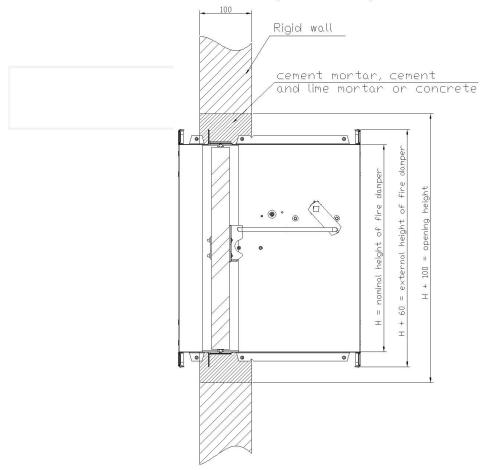
Figure 6 Installation method of fire dampers KWP-L in rigid wall
