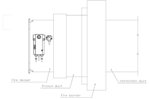
Figure 13. Installation of fire dampers KWP-L away from wall construction according to point 2
