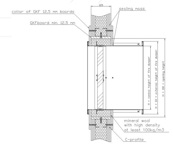
Figure 11. Installation method of fire dampers KWP-L in flexible wall 125 mm thick
