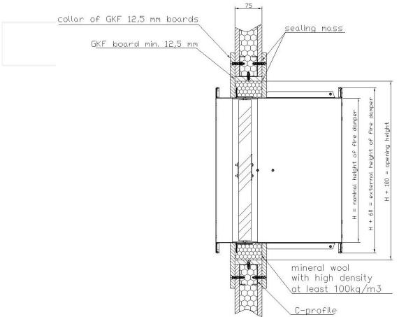
Figure 9. Installation method of fire dampers KWP-L in flexible wall 75 mm thick
