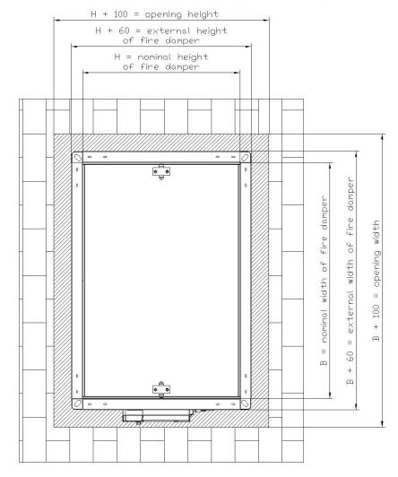
Figure 4. Installation method of fire dampers KWP-L in rigid wall with vertical rotation axis of baffle
