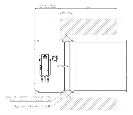
Figure 12. Installation method of fire dampers KWP-L in constructions of great thickness
