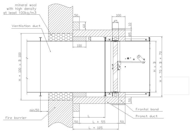
Figure 14. Installation of fire dampers KWP-L away from wall construction
