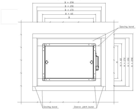
Figure 15.Installation of fire dampers KWP-L away from wall construction
