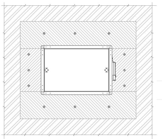
Figure 8. Installation method of fire dampers KWP-L in flexible wall with horizontal rotation axis of baffle
