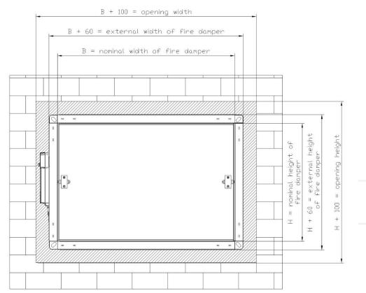
Figure 5. Installation method of fire dampers KWP-L in rigid wall with horizontal rotation axis of baffle
