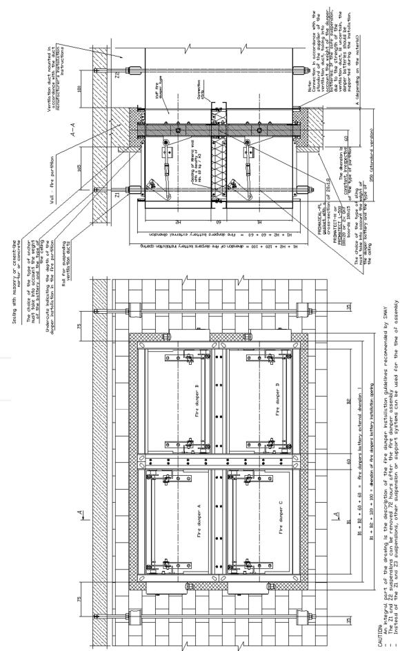
Figure 19. Installation of a battery consisting of four fire dampers KWP in wall
