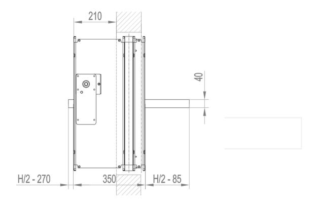
Figure 10. Dimensions of the building partition depending on the high of a damper
