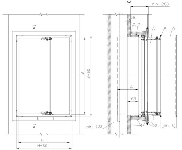
Figure 9.Installation method of dampers on the tee
