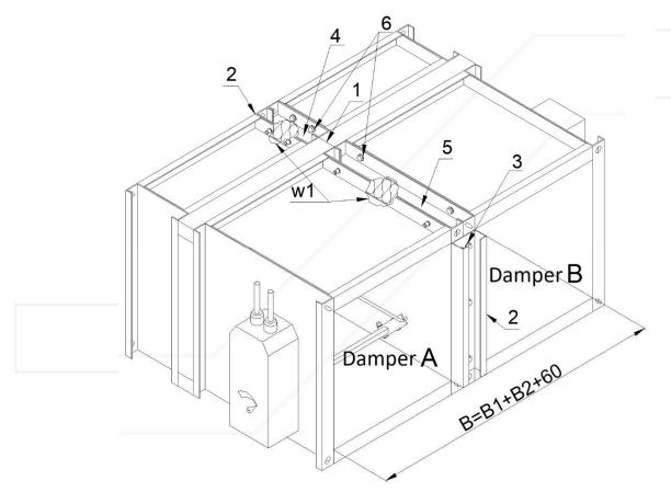
Figure 14. Arrangement 3 - horizontal battery consisting of two fire dampers KWP
