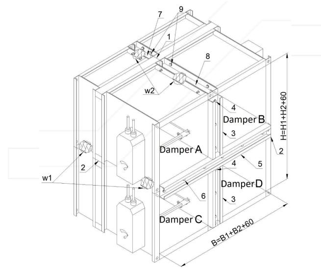
Figure 15. Battery made of four dampers KWP-O
