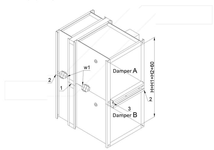
Figure 12. Arrangement 1 - vertical battery consisting of two fire dampers KWP
