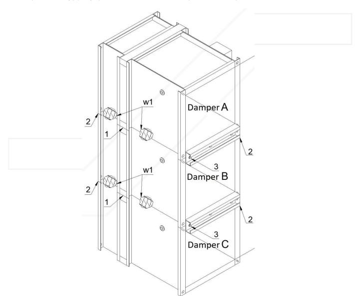
Figure 13. Arrangement 2 - vertical battery consisting of three fire dampers KWP
