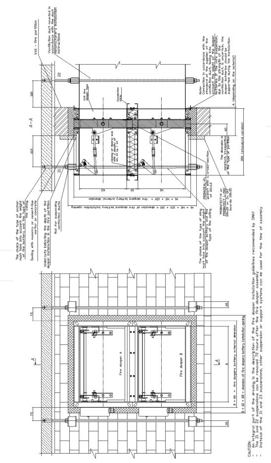
Figure 16. Installation of a battery consisting of two fire dampers KWP in vertical arrangement in wall
