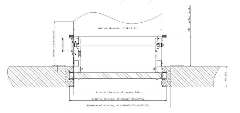
Figure 6. Installation method of fire dampers KWP-O in ceiling with a fire ventilation duct with sealing of cement
