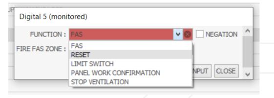
Figure 4.6 Available functions of a monitored digital input.
