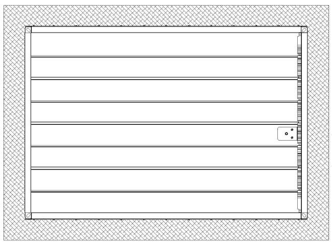
Figure 8. Installation method of fire dampers WKP-O in standard wall
