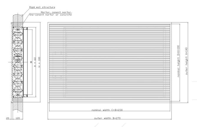
Figure 11. Installation method of KST grille
