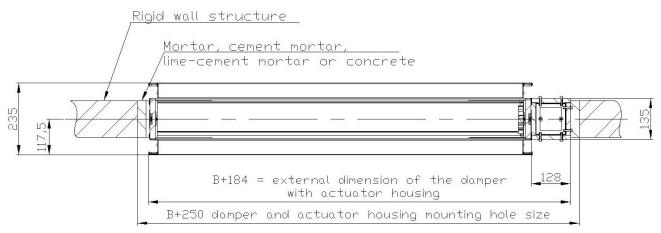
Figure 3. Installing method of WKP-O fire dampers in rigid wall
