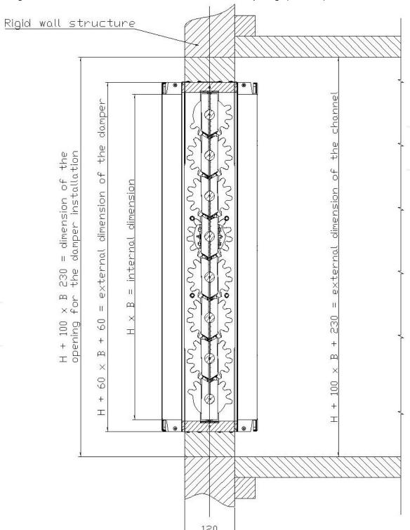
Figure 5. Installing method of WKP-O fire dampers with PROMAT boards duct.
