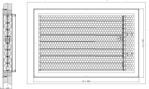
Figure 9. Installation method of MKW-B honeycomb mesh cover
