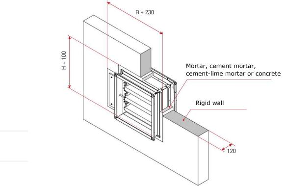
Figure 1. Dimensions of the installation opening of the WKP-O dampers in rigid wall with a horizontal and with vertical axis of rotation of the baffle, with planned cut for actuator housing. The C dimension is given in the table.
