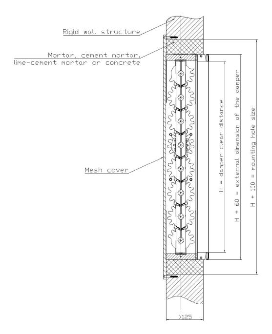
Figure 6. Installation method of fire dampers WKP-O in structures thicker than 125 mm
