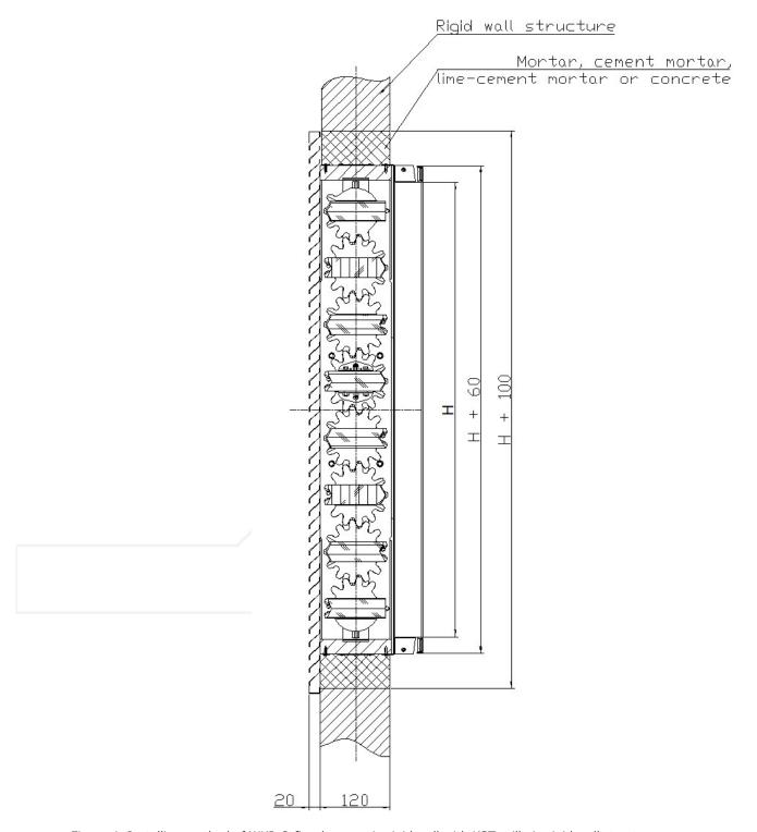
Figure 4. Installing method of WKP-O fire dampers in rigid wall with KST grille in rigid wall structure.
