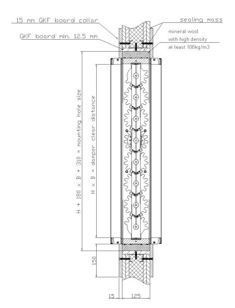
Figure 7. Installation method of fire dampers WKP-O in standard wall with 125 mm thick
