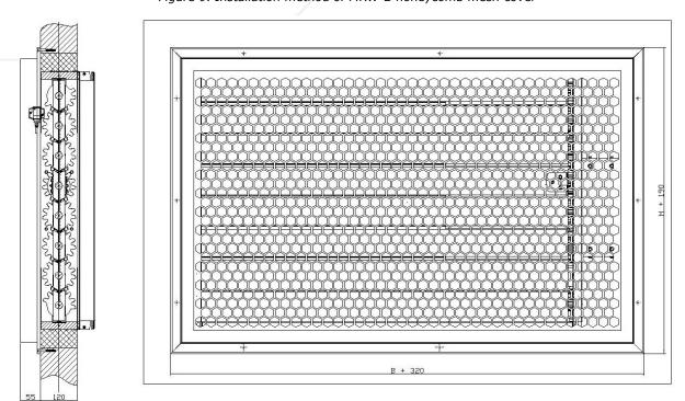
Figure 10. Installation method of MKW-D honeycomb mesh cover
