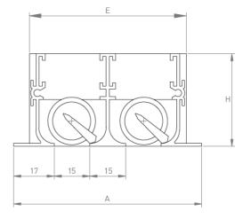
Figure 2. Dimensions of NSAL-70 front panels
