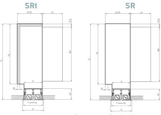
Figure 4: Dimensions of plenum boxes for NSAL-70
