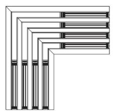
Figure 5. Sketch of the corner connector.
