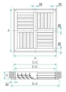
Figure 1. NWC front panel dimensions.
