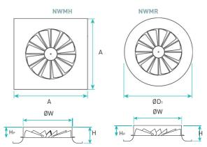
Figure 1. Dimensions of the NWMH/NWMR diffuser front panel.
