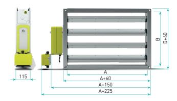
Figure 1. PWIIS-EX damper dimensions.
