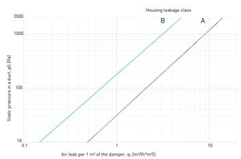
Chart 3. Air leaks through the PWIIS-EX damper housing (in a fully closed
