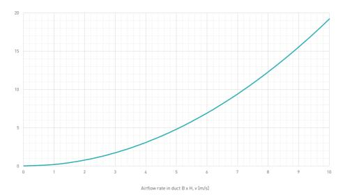
Chart 1. Pressure loss for a standard-height PWIIS-EX damper (in a fully open position).
