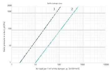
Chart 2. Air leaks through the PWIIS-EX damper baffle (in a fully closed position).
