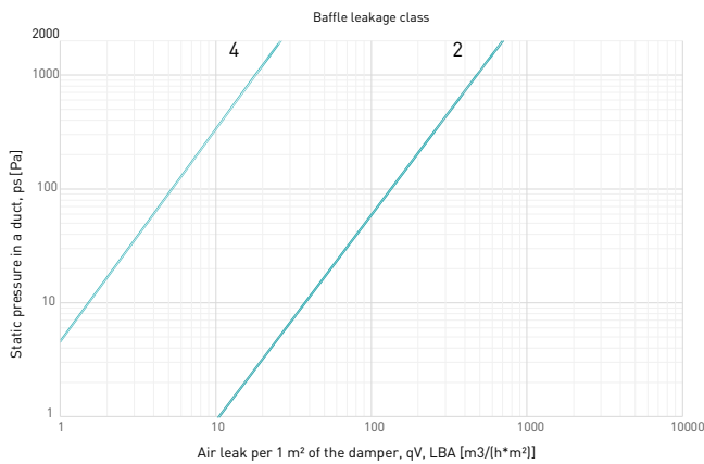
Chart 2. Air leaks through PWIS-N damper baffle (in a fully closed position).
