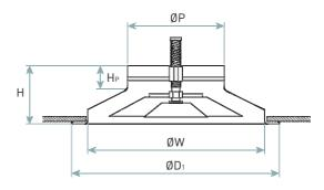
Figure 3. SDRW diffuser dimensions.
