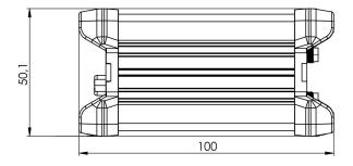
Figure 1. RUT 955/956 Router Dimensions.
